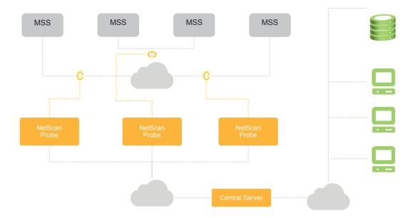
NetScan monitoring system passively intercept data (signalling & UP) from monitored network and process at NetScan Probes. All probes are fully autonomous and continue data processing even with no contact with other system components (central server, other probes).
