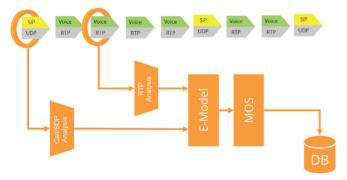
RTP-based voice quality analysis does not require actual voice decoding to score quality. The only information needed is type of the codec used as it is required by E-model to calculate R-factor. Codec information can be taken directly from RTP (for those codecs using predefined PT value) or from control plane monitoring (typically – SIP).
